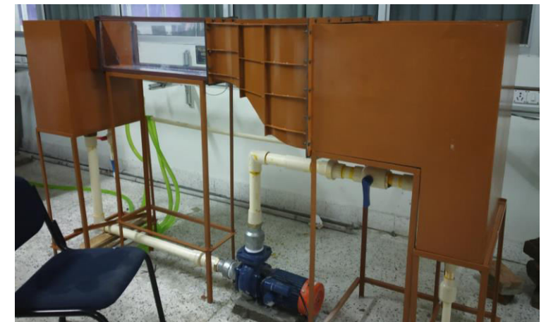
A 20 X 20 cm 2 test section water tunnel designed and fabricated at IITG
